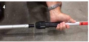
Insert the threaded tip of each extension pole into the collared receiver at the bottom of the net pole. Twist the extension pole to screw it onto the net pole. Tighten the collar to lock the parts firmly in place. Make sure the collar is unscrewed all the way before screwing the pole into it.
