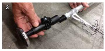
Attach the appropriate head (magnet or hook) to the end of each net pole top by screwing them onto the threaded tip.
