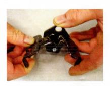
To set your BOOGER retriever, simply open the fingers while using your thumbs to insert the "ears" of the spring trigger into the holes on each side. You will hear a click when correctly set and the fingers will remain open. When retrieving an object, simply drop the BOOGER on it; the trigger will release and the fingers will grasp it. The BOOGER retriever works effectively on any dropped item. Use a strong nylon or braided cord for optimum control.
