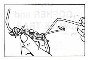
3. Slide flat metal trigger piece toward jaws with the points up. Put long end of the tail that is resting on the spring through the hole of flat metal trigger.
