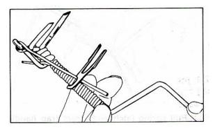
4. To set trap hold trap handle in right hand, and catch spring latch with left thumb and place two fingers under the spring (as shown in the drawing). Hold firm cranking the trap handle to the right until the spring latch meets the trap handle and is latched to the trap handle.
