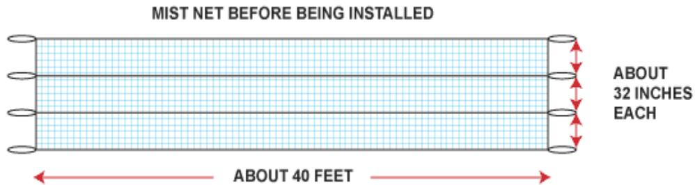
By raising loops 2, 3, 4 and 5 on each side, you create pouches (or pockets) that the birds tumble into after hitting the net. Birds that hit the net don't typically get entangled. After hitting the net they lose air speed and usually tumble into the pouches created during installation.
