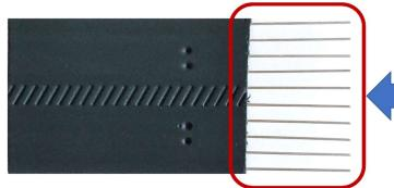
The rodent proofing barrier consisting of 10 solid wires of stainless steel with a diameter of 1/25 in (1 mm) stripped from the thermoplastic vulcanizate. The spacing between the wires is 1/5 in (5 mm) – too little for a mouse to squeeze through.
