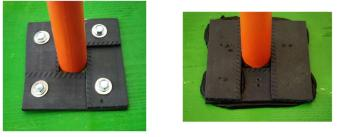
A single layer is normally sufficient. A double layer can be installed if the rodent pressure is very high or if a particularly high degree of protection is required. A single layer can proof up to 1.4 in (3.5 cm) wide gaps. A double layer can proof up to 2 in (5 cm) wide gaps.
