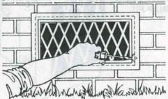
7. IF A RETAINING SPRING HAS TO BE MOVED FROM ONE SLOT TO ANOTHER OR NOT USED AT ALL, PLIERS SHOULD BE USED TO EXTRACT THE RETAINING SPRING. FORCE IS REQUIRED AND DOING THIS BY HAND IS NOT RECOMMENDED.
