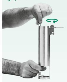
Bring the rocker into locking position (see page 25). Bring the two triggers, one after the other, in position and hold them there with one hand. Grasp the small hook of the snapper arm and turn clockwise until the hook and triggers are positioned parallel to the rocker.
