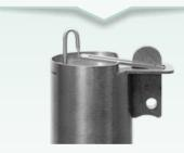
Slowly release the rocker, until the tip of the rocker touches the tip of the snapper arm.
