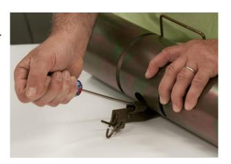
4) After adjustments you may have to loosen the nut and bolt to the pan to make sure the pan moves easily and isn't tight.
