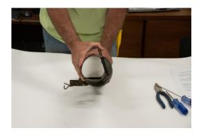
To fix a bend, put a broom handle or similar size bar through the trap on the dog and safety side, between the strike bar and inside of the tube trap. Lightly push the top of the strike bar toward the broom handle you have inserted into the tube trap, pushing lightly until the strike bar has been straightened.
